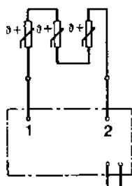
Semiconductor temperature detector with release
