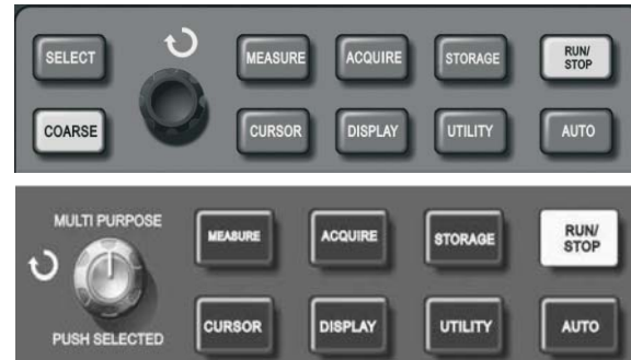
Figure 2-29 Function key (or cursor) of sampling system
