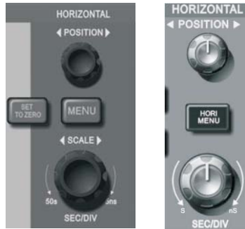
Figure 2-11 Interface of horizontal system
