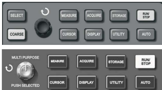
Figure 2—27 Function key (and function) of sampling
